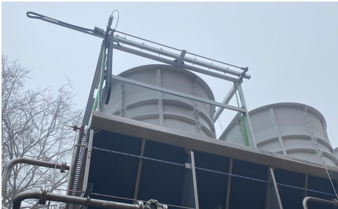
Figure 1: Hybrid cooler MoNiKa and velocity and temperature sensors at the diffuser outlet
